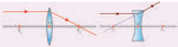
Figure 2.4 Rays passing parallel to the optic axis
