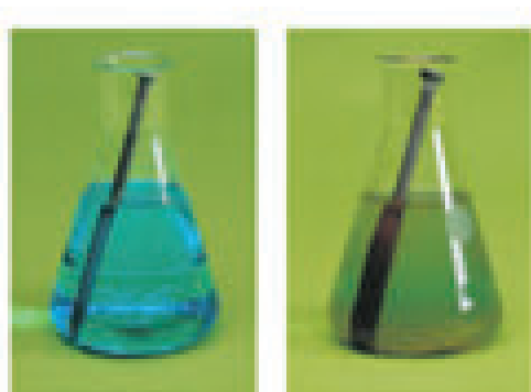
Figure 10.2 Displacement of copper
