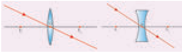
Figure 2.3 Rays passing through the optical centre
